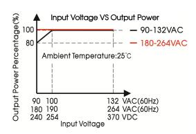
Note: 1. With an AC input voltage between 90-100VAC and a DC input between 180-190VDC the output power must be derated as per the temperature derating curves;
