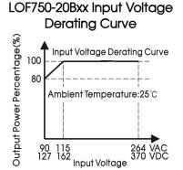
Note: With an AC input voltage between 90 - 115VAC and a DC input between 127 - 162VDC the output power must be derated as per the temperature derating curves.
